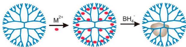
SCHEME 6. Crook's Synthesis of a Nanoparticle inside a PAMAM Dendrimer a
